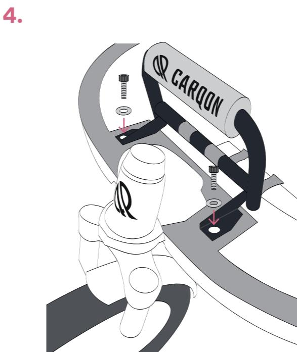
**EN** Place the headrest on the front frame of the Carqon Cruise, so that the belts fall into the box and the side supports go over the points to attach the bolts (M10): The recommended tightening torque is 24 Nm. Advice: use an Allen key 8 to tighten the bolts.
